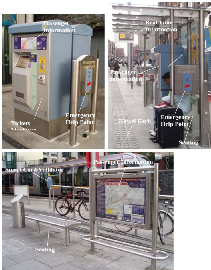
Figure 9.2 Typical system characteristics, LRT (Dublin)
